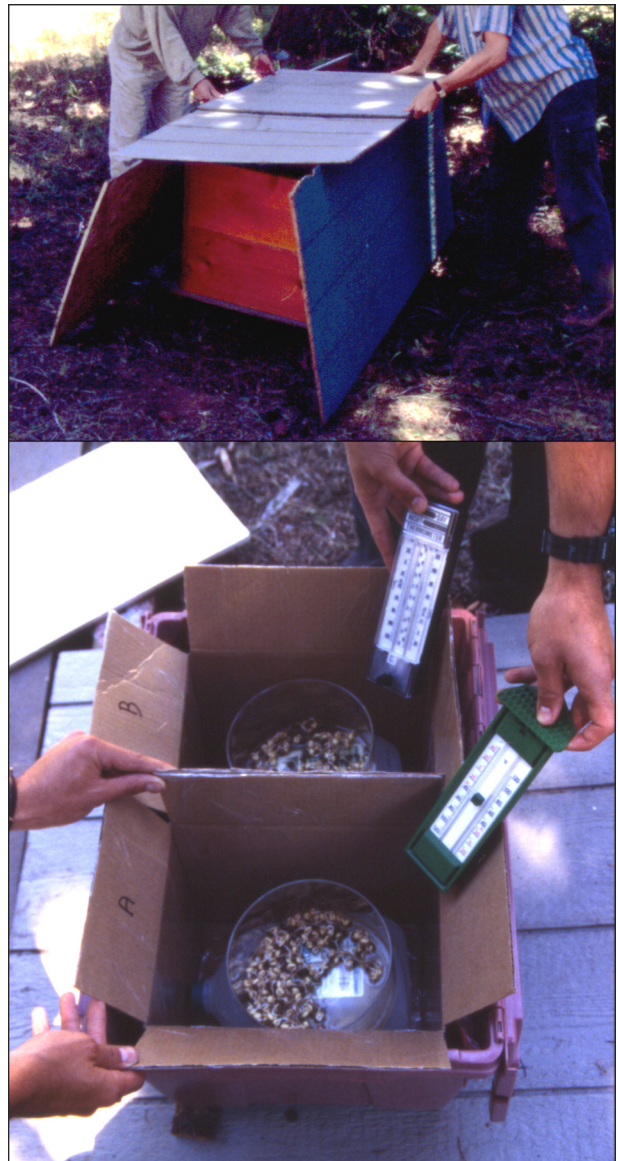
Figure 2. The Control Enclosure: Control seed dishes were kept inside a cardboard box along with max-min thermometers (below), which was in turn nested inside an insulated plastic box, placed on an elevated platform under a heavy wood box, with shade panels added (above), under a forest canopy. Adjustments to ventilation and shading allowed the temperature within the control and orgone accumulator enclosures to be adjusted very close to each other.
