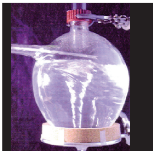
Figure 21. Hyperbolic vortex created by tangential water flow in an egg-shaped glass container
